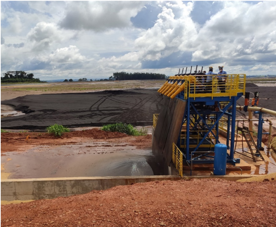
Figure 1: Magnetic tailings cycloning.
