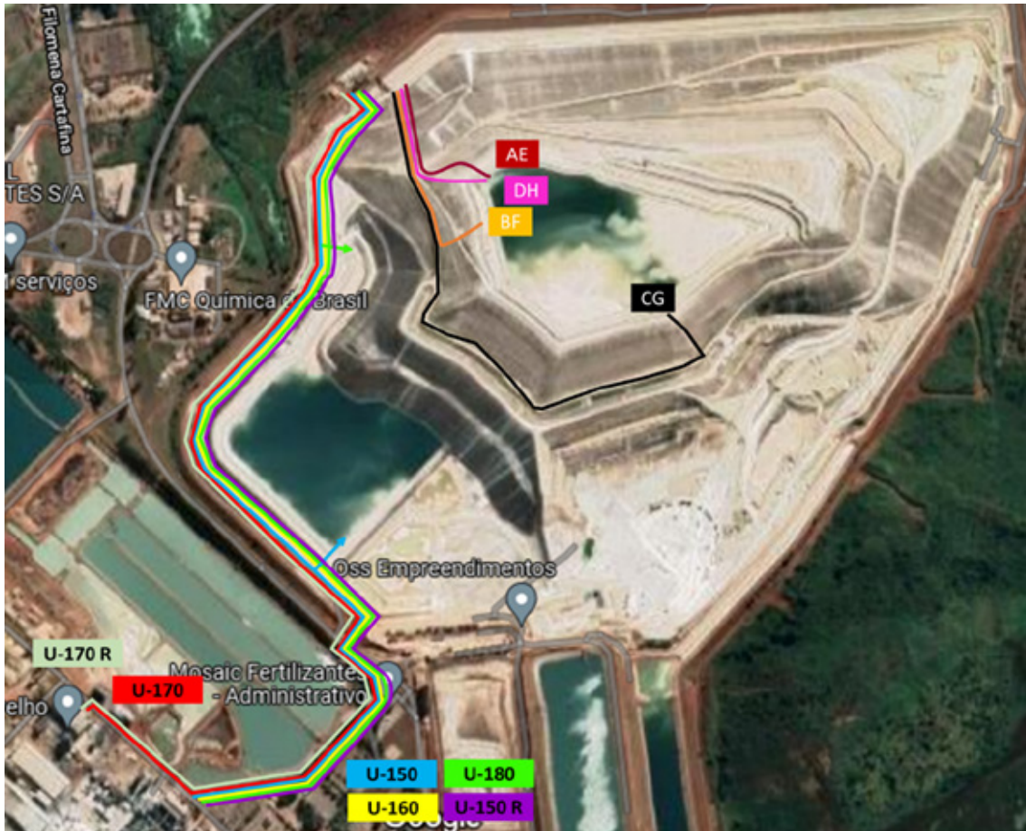
Figure 2: Air view of gypsum pile and existing gypsum pumping lines (Mosaic Fertilizantes)
