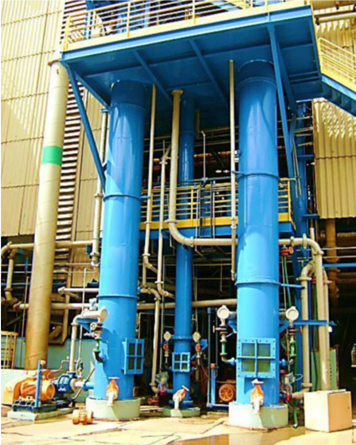
Figure 1: Flotation circuit view for barite concentration..
