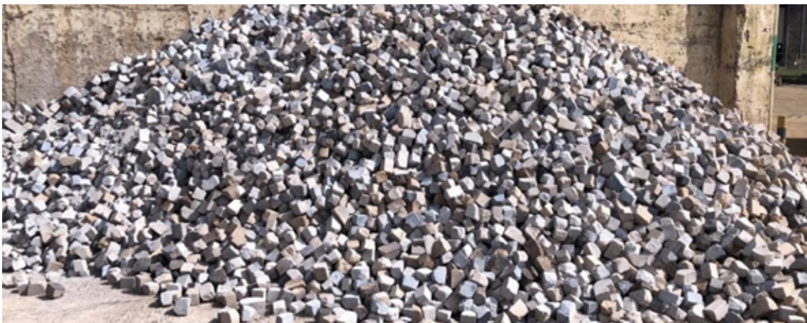
Recovered refractory brick photo
