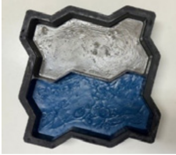
Geopolymer interlocked floor piece.
