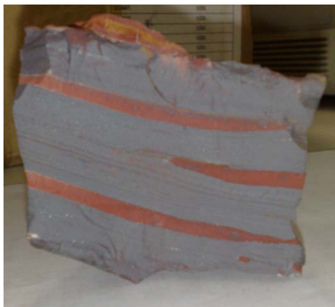
Figure 3 – Detail of interleaved layers of silica and iron ore in jasper, contaminated by P. [1]
