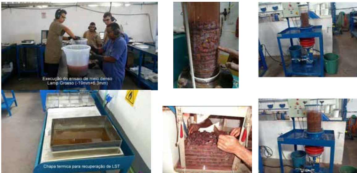
Figure 4_1 – Photos of the left side: Geomatek Laboratory - Tests with LSD; photos of center: jigs of Fundação Gorceix; photos of the right side: jig for bench tests of HD drill cores samples
