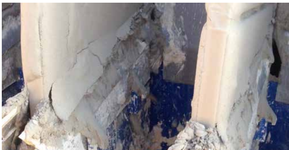
Figure 8 – CX-Series, Filter Cake Production and Discharge (March 2016)
