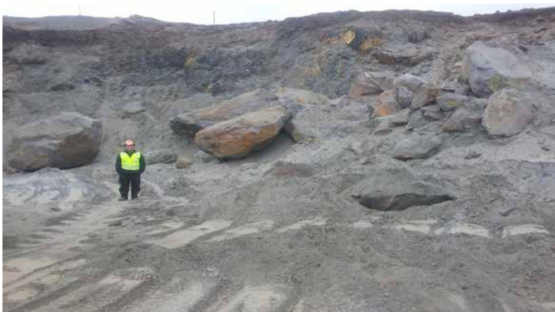
Figure 1 – Oversize material (boulders and blocks) of hard itabirite preserved after regular blasting. The boulders are amid soil and highly altered rocks.
