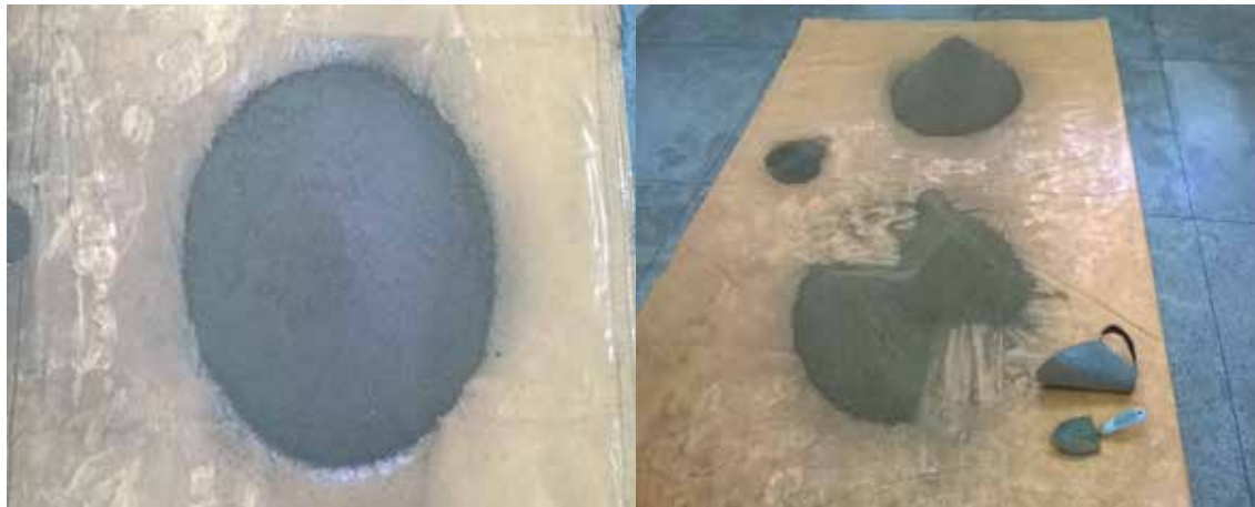
Figure 1- Procedure for homogenization and quartering samples.
