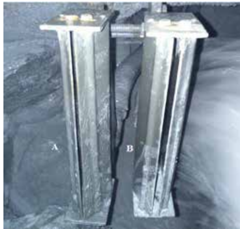
Figure 1 – Falling stream cutters (A – reference cutter; B – experimental cutter) sampling the final tailings stream
